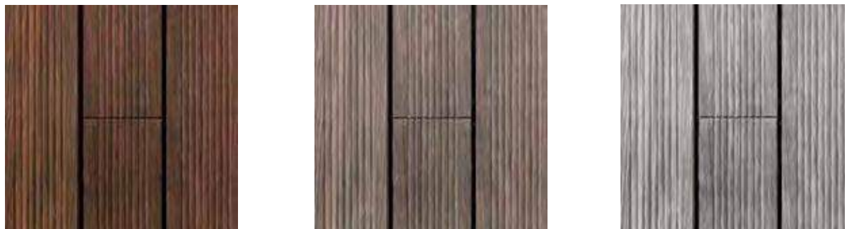
Gradual greying of Bamboo X-treme® over time: new, non-weathered decking (left), after 3-6 months of weathering (middle) and after 18 months of weathering (right) - without oiling.
